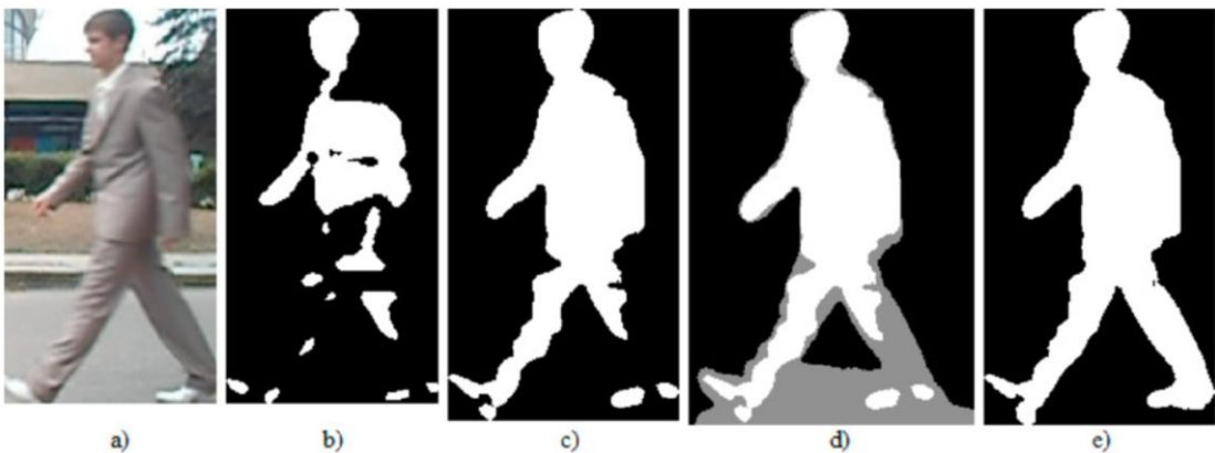
Different parameters KNN-based Background/Foreground segmentation algorithm results: (a) original image; (b) History = 500, Dist2Threshold = 400, \tau = 0.5 ; (c) History = 200, Dist2Threshold = 30; (d) with shadow; (e) \tau = 0.75 .
